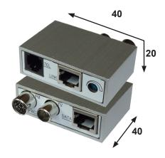
Triple-play adapter to connect a TV set, a digital settopbox and an FM tuner to a universal OmniMedia RJ45 wall outlet using a standard RF coax and RJ45 patchleads.
